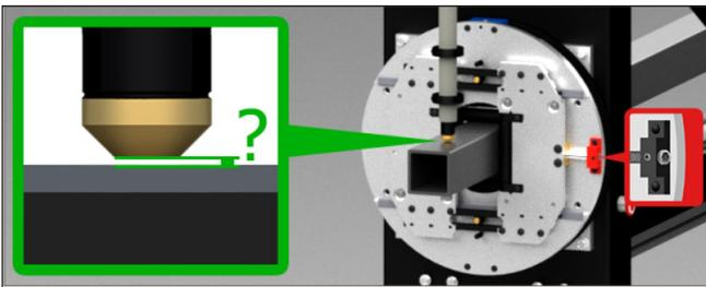
The program will ask the Operator to record the gap distance between the Torch and the material for each side of the material. This can be accomplished using a set of feeler gauges and Vernier calipers. Before beginning, verify the Gate Lead Screws are in the 12 o'clock and 3 o'clock positions.
