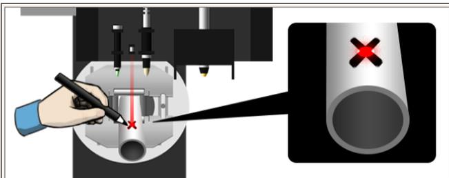
The program will ask the Operator to move the Laser. This will move the Laser to the center of the material.
