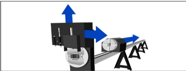
The Operator will be asked to perform the machine's Homing process. To begin the Homing process click the image in the interface.
