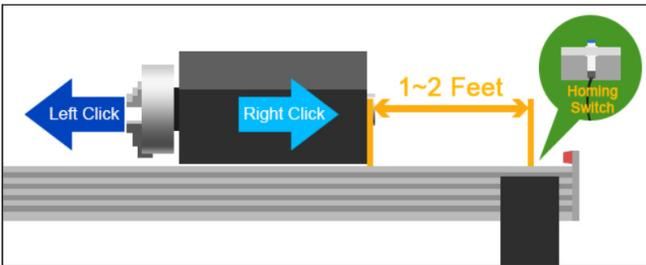
The computer will ask the Operator to use the mouse to jog the Trolley within 1-2 feet of the end of the Rail.
