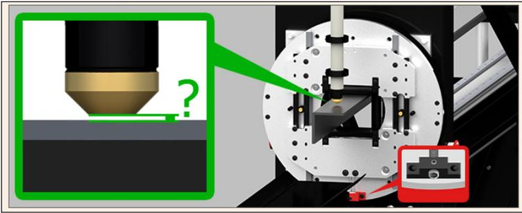
The program will ask the Operator to record the gap distance between the Torch and the material for each side of the material. This can be accomplished using a set of feeler gauges and calipers as outlined in section 1.1.7.
