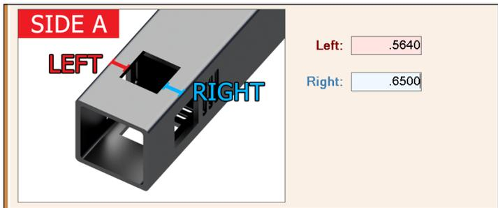
The program will ask the Operator to measure the distance of the left hand and right hand side of the hole to the edge of the material.
