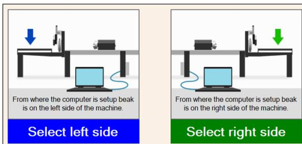
The procedure will then ask the Operator to choose a left side and a right side of the machine based on where the operator has placed the computer. Choose which side the computer is placed.
