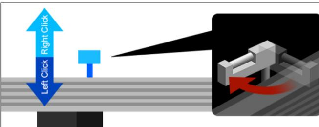
The Lifter Station Switch establishes the the engagement position for the Material Support Lift.
