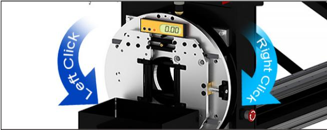
Calibrating the Powered Gate requires the Operator to place a level on the Gate. As indicated on the screen, the best place to do this is by placing the level on the top of the front adjustable Gate as shown in the image on the screen. Use the right and left mouse buttons to jog the Powered Gate into a level position.
