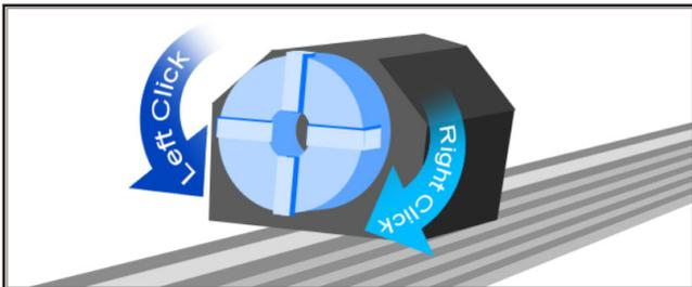
The program will then ask the Operator to verify the Chuck is moving properly in relation to the computer mouse controls.
