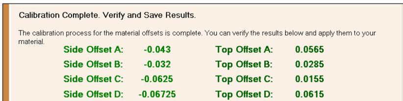
An interface will open showing the Side Offset values for the material. The program will use the material size and the values entered in the Side Offset Calibration to center the holes on each side.
