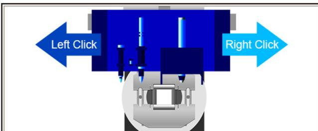
Next the program will ask the Operator to use the computer mouse to verify the Toolhead is moving properly from side-to-side.
