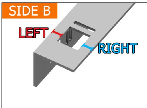
The program will ask the Operator to measure the distance of the left hand and right hand side of the hole to the edge of the material. Use the images on the interface as a reference regarding which sides to measure.
