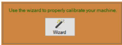
From the home interface, open Bend-Tech CAM software. Open the Machine Control interface. From the Tools dropdown, click Machine Library, select Dragon, then click the Wizard icon.
