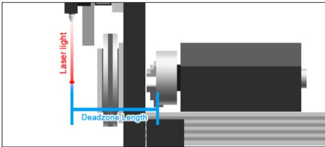
However, the Dead Zone is subjective and can vary between machine and Operator depending on the Maximum Chuck Travel procedure.
