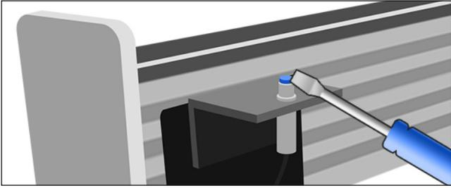
Homing Switch operation is checked by touching the face of each switch with a metal tool, such as the blade of a screwdriver.
