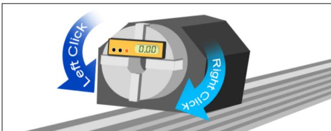
Calibrating the Chuck requires placing a small level or angle finder on the Chuck teeth. Once the level or angle finder is placed, the Operator can jog the Chuck into a level configuration using the left and right mouse buttons. With the Chuck head calibrated to level it is now synchronized with the Toolhead. This is critical when performing cutting procedures.
