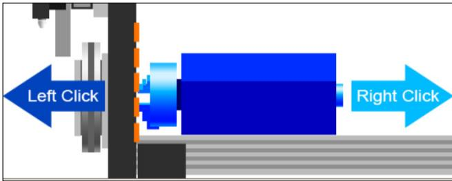
Max travel length is determined by moving the Trolley as far forward as possible. It is recommended that the Operator move the Trolley forward so there is a minimal amount of space visible between the front surface of the Chuck teeth and the Toolhead when viewing from the side of the Toolhead. If there is no space visible the Trolley is too far forward.
