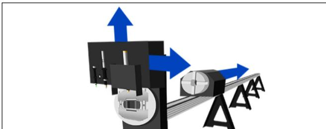
The program will then ask the Operator to click the image on the screen to begin the homing process. Click the image. A message will appear informing the Operator that the machine is homing. Click Next after the message disappears.
