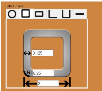
Select the shape of the material that will be used in the Select Shape box on the right hand side of the interface. Enter the dimensions of the material in the appropriate text boxes. Enter a name for the material.
