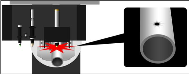
Click the Pierce Hole button to initiate the Torch action. The Torch will move to the material and fire once. Depending on what the machine amperage is set at the Torch may only gouge a hole, it may not pierce through the material. This is sufficient for calibration purposes.
