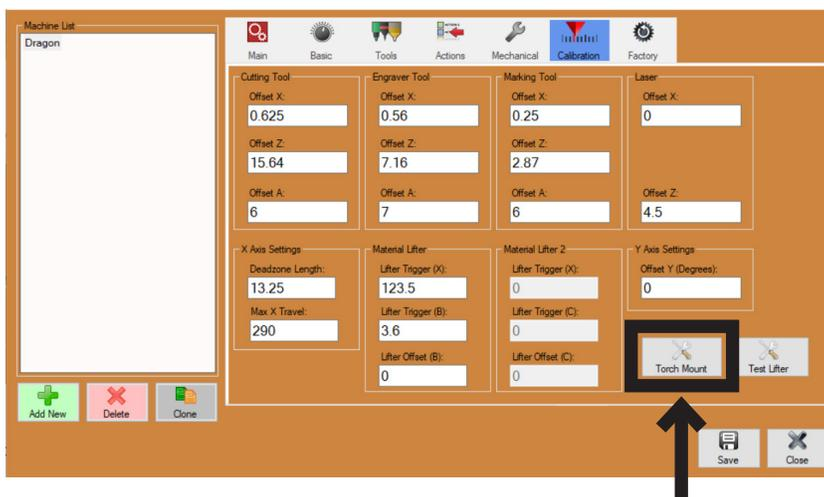
Click Torch Mount at the bottom right of the new interface. This will open the Torch Mounting Utility interface.
