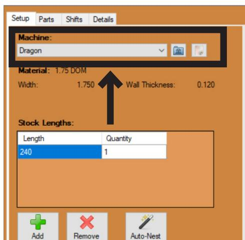
The Operator will choose a machine where the Nest Part project will be run. The Operator will have already chosen a name for the machine as outlined in Chapter 3 of the Start-Up and Training Manual Part 2. Most shops will only have one Dragon A400 machine logged into the computer, in which case it will default to that machine.
