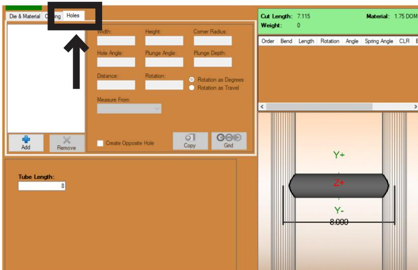
Click the Holes tab. The Holes interface allows the Operator to choose and set up a variety of holes that can be cut into the material.
