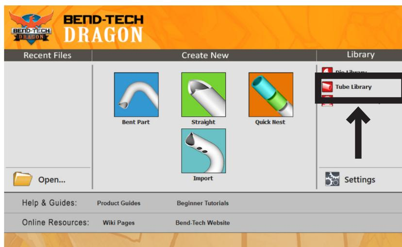
Before performing any type of cutting procedure on the Dragon A400 the Operator must first add material(s) into the Tube and Pipe Library.
