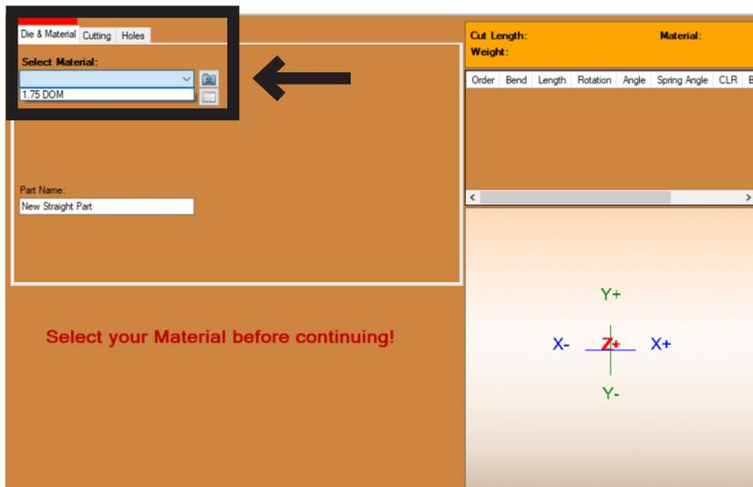
Select the Die & Material tab near the top left of the interface. In the pull down menu choose the type of material you will be working with from the Tube and Pipe Library. Refer to Chapter 2 of this section to see how to enter material into the Tube and Pipe Library.
