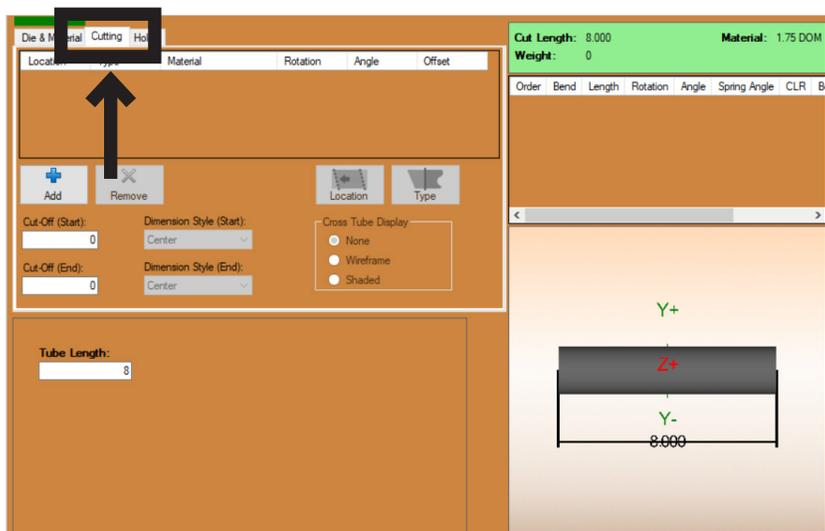
Click the Cutting tab. The Cutting interface allows the Operator to choose and set up a variety of cuts on the material.
