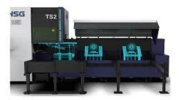
The unloading positions are equipped with one follow-up flip plate and two follow-up concave wheels that can move forward and backward and rise and fall. The position can be intelligently adjusted according to the length of the workpiece, providing stable support during cutting and unloading processes.
