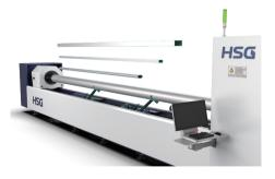
Its advanced digital intelligent dual chuck and independent servo follow-up support, engineered for versatility, the TS2 series standard configuration includes two clamps for tubes and profiles, capable of processing tubes with a weight of  $\leq$  300kg(661lbs). It supports cutting profiles such as channel steel, angle steel, and H-beams.
