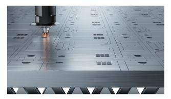
With high-power output, the GV Series machine significantly increases the efficiency of cutting medium-thick plates. With a 60kW system, it provides cutting speeds that are up to 400% faster than traditional 12kW systems, resulting in increased output per unit time and reduced cost per piece.
